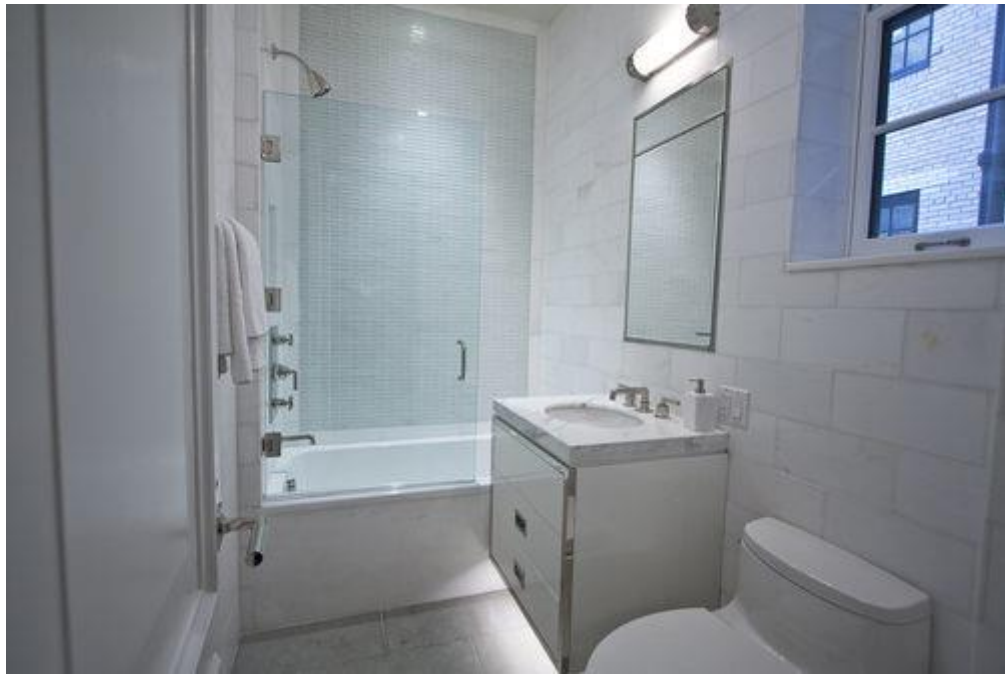
Floating glass shower door is spring-loaded in the hinges so it returns to this position.
